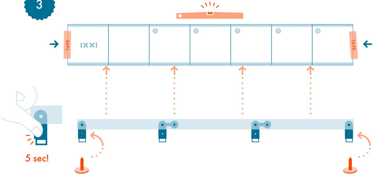
Attach this manual (help for hanging) to the wall with tape, level and dead straight, on the spot where you want to hang the IXXI.
