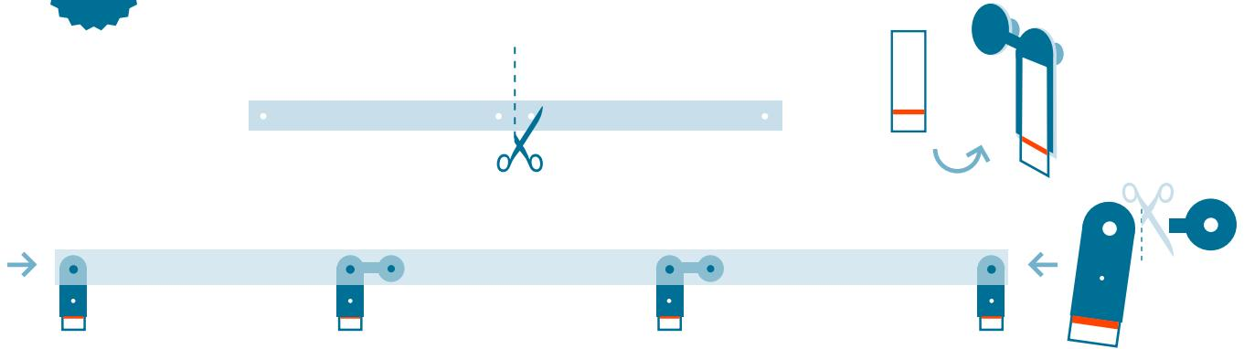
Cut the strip to the width of your IXXI. Attach the Power- strips to the backside of the Monos, and click it into the strip.
